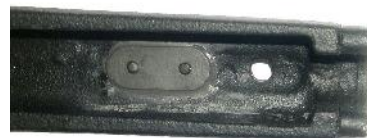
Inside View: Nut Plate epoxy bedded to USGI fiberglass stock
