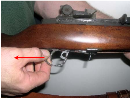
Fig 1 - Pull Trigger Guard Toward Rear to Unlatch
