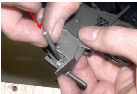
Fig 10 - Use Taper Pin Inserted In Left Side to Align New Mag Latch
