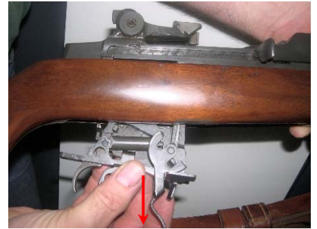
Fig 3 - Pull Trigger Group Straight Down
