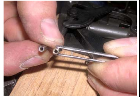
Fig 15 – Old Split Pin on Left New Medium Coil Pin on Right
