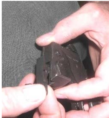
Fig 8 - Remove Old USGI Mag Latch
