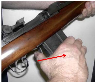
Fig 23 – Removing Magazine Using Newly Installed Mag Latch
