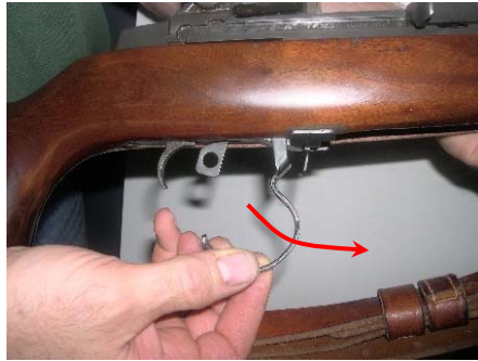
Fig 2 - Pull Down and Swing Out
