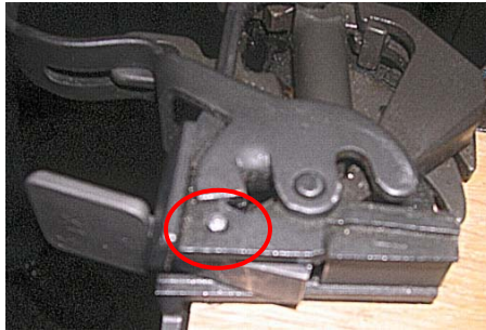
Fig 14 – Small End of Taper Pin Shown Protruding on Right Side of Trigger Housing
