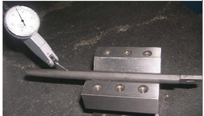
Every Sadlak Spring Guide is individually inspected for straightness within .002
