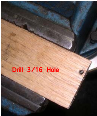
Fig 4 - Make Wood Block with 3/16 Drilled Hole located 5/32 from End (See Attached Drawing)
