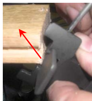
Fig 11 - Compress Spring Using Corner of Wood Block and Align Housing and Mag Latch Hole
