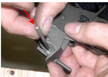
Fig 10 - Use Taper Pin Inserted In Left Side to Align New Mag Latch
