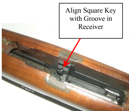
Fig 20 – Align Square Key in Trigger Housing with the Sq Groove in the Receiver
