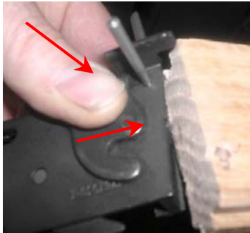
Fig 13 – Insert Taper Pin on Left Side to Keep Parts Aligned
