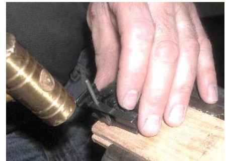
Fig 6 - Taper Pin Shown Fully Inserted with Pivot Pin Driven Out Thru the Hole in Wood
