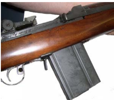
Fig 22 – Completed M1A with New Tactical Magazine Release Latch
