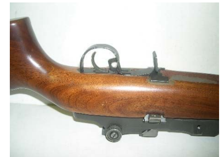
Fig 21 – Insert Trigger Group Until Flush to Stock and Snap Trigger Guard Closed
