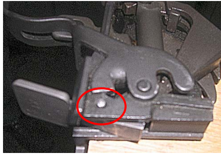
Fig 14 – Small End of Taper Pin Shown Protruding on Right Side of Trigger Housing
