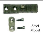
The <u>Steel Model</u> with the optional QD Stud shown at the left takes advantage of the Sadlak Internal Oval Nut plate (as used on our QD Post Assembly) using two socket head screws installed externally through the two counterbored holes in the rail. This model allows the removal or replacement of the rail without removing the stock. Depending on the stock, initial installation of the internal nut plate may require Dremel work to recess the oval plate flush to the inside surface.
