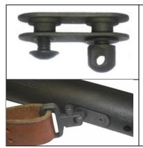
The Sadlak QD Post replaces the stock M1A/M14 front swivel for a more rugged, durable bi-pod attachment. It eliminates cracking of the stock during heavy recoil or rough use. The internal oval nut plate and external oval washer has approximately 3 times the load disbursement over the standard single Quick Disconnect (QD) post
