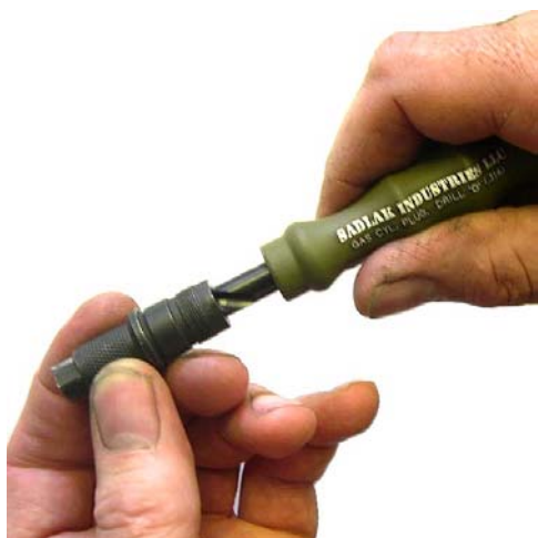
Gas Cylinder Plug Cleaning Drill - Letter "O" Drill (Dia .316)
