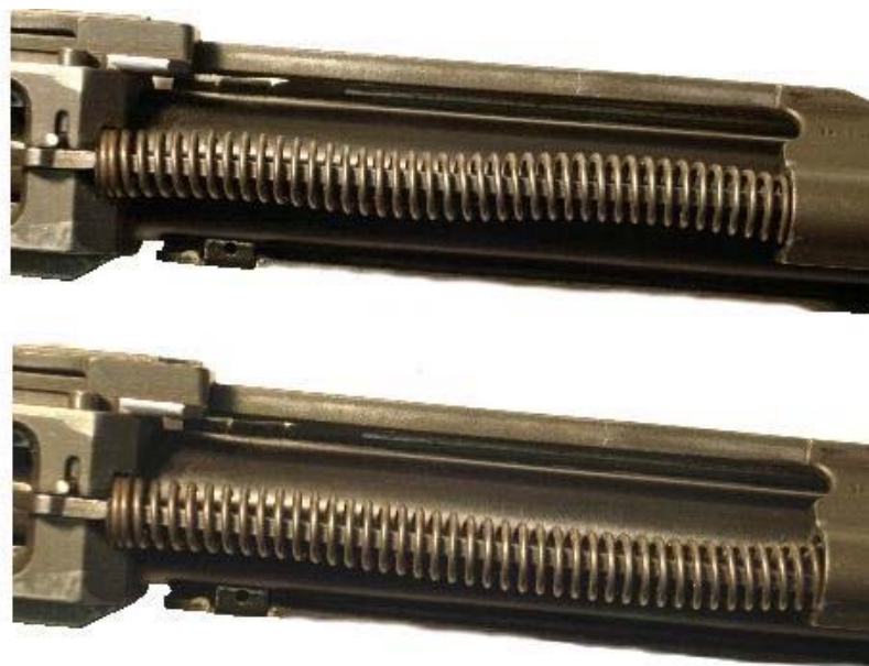
Fig 3 USGI Spring Guides Installed
