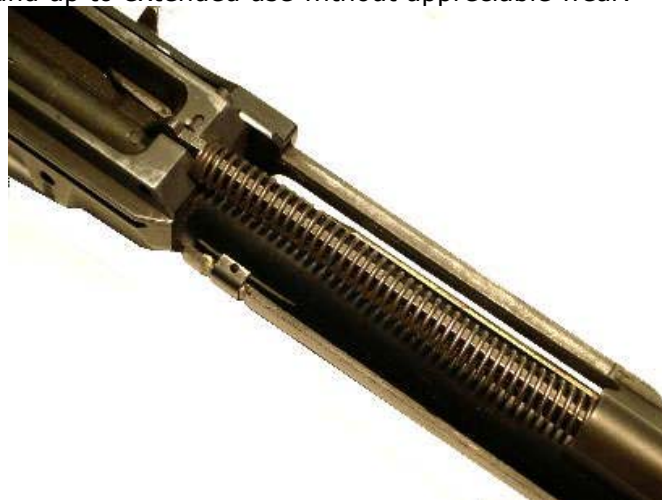
Fig. 8 Sadlak NM Spring Guide Installed
